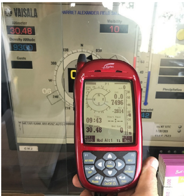
Figure 1: Instrument set to precise QNH altitude
